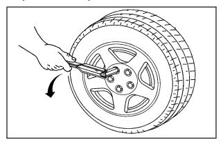
To remove the steel wheel covers and wheel nut caps, loosen the plastic nut caps with the wheel wrench in a counterclockwise direction.
